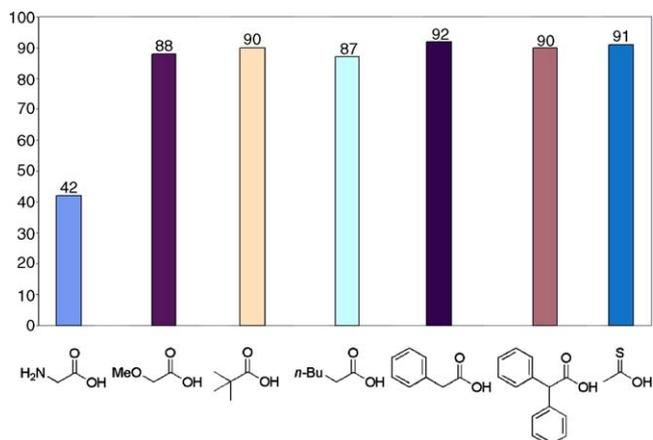
Fig. 2. Plot % conversion to cyclooctene oxide obtained using various substituted acetic acid derivatives, after 4 h reaction time, in the presence of  $\text{Na}_2\text{WO}_4/\text{H}_2\text{WO}_4/\text{Aliquat 336}/\text{H}_2\text{O}_2$  at  $60^\circ\text{C}$ .
